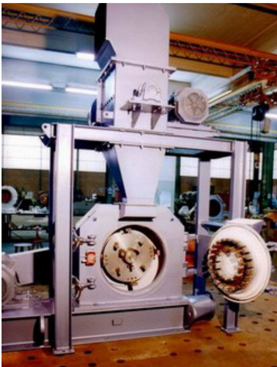
Crusher set on top of a Duplex 25 AME Mill feeder, set for the pre-milling function.
