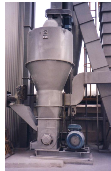
MS 70 mill in milling of calcium carbonate.
