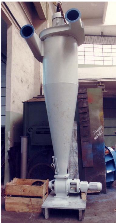
Cyclone with fan and alveolar valve for discharge.
