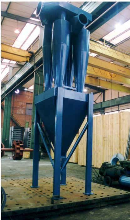
Cyclonic group composed of four cyclones, common hopper discharge and support legs.
