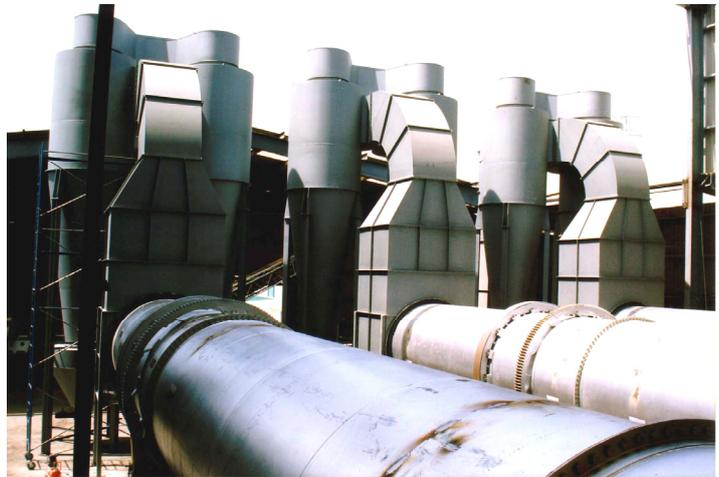
Installation of cyclones in industrial process.
