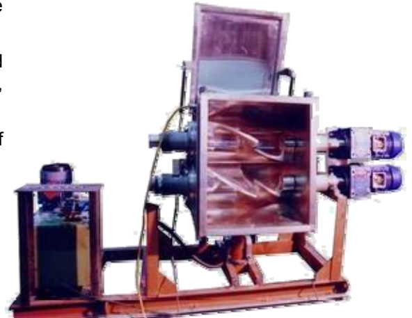
Kneading machine ZETA 500, in stainless steel.
