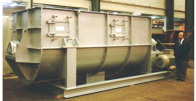
Mixer ME-800 of 8.000 l of capacity, made in carbon steel
