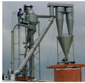
The high efficiency cyclone equipments are the most commonly used equipments in dust separation processes or materials in suspension in an air stream.
